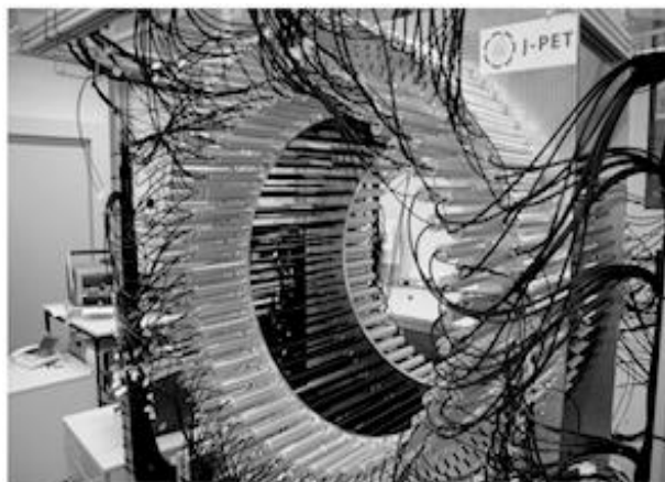
Fig. 1. The first full scale prototype of the J-PET scanner. Plastic scintillation strips (black) are visible, as well as photomultiplier tubes (grey) (Niedzwiecki et al. 2017).
