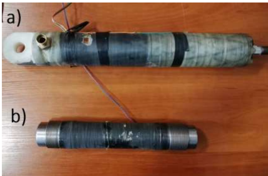
Fig. 2. Prototypes of hydraulic cylinders made of composite materials: a) – full cylinder made of carbon fiber, polymers and metal alloys; b) – cylinder barrel made with a steel liner and CFRP hoop reinforcement
