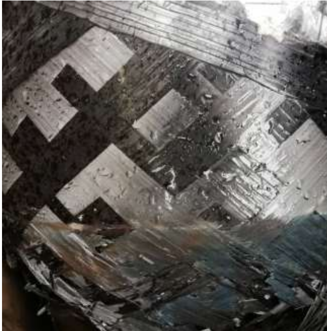
Fig. 5. Example of the crossovers between layers of carbon fiber in the element made by filament winding process
